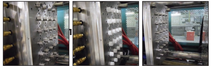
With DT Cores, no hydraulics or external core pull mechanisms are required.
